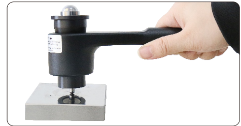
Hammer impact to apply test force
