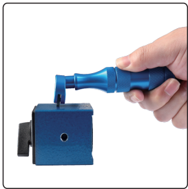
step 1: make grid cutting on surface
