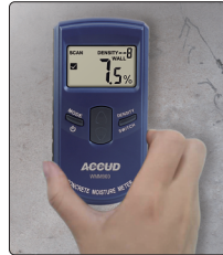
Measure concrete moisture
