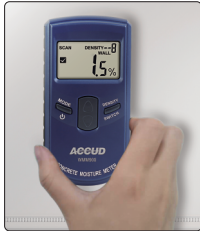
Measure wall moisture
