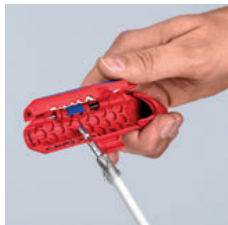
Stripping of a coax cable
